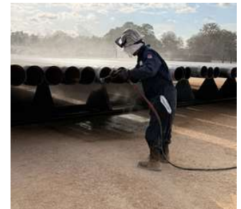
On the rack: working box ends, and cleaning casing ahead of inspection.
