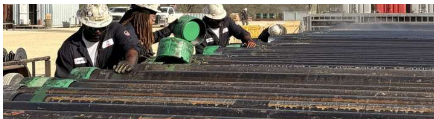
Our crew pulling thread protectors on the rack, in full PPE.
