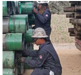
On the rack: working box ends, and cleaning casing ahead of inspection.
